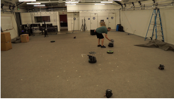
(a) Heterogeneous team of differential drive robots navigating through an environment without obstacles. A person changes the positions of the robots while RLSS is running.
